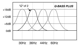
**CAUTION:** *QBASS PLUS*<sup>™</sup> should only be used in systems with a strong subwoofer section. +18dB is a tremendous amount of bass boost and may damage your speakers or create excessive distortion if abused.
